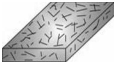
Gambar 2.7 Serat Chopped Strand Mat. (Gibson, 1994)
