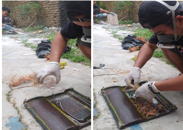
Gambar 4.9 (a)Penuangan Resin (b)Pemberian Serat.
