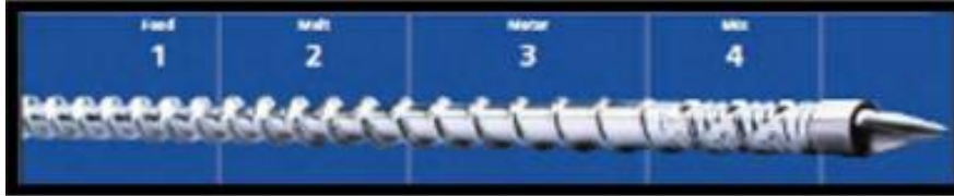
Gambar 2.9 barrel screw (Singgih kurniawan/2010)
