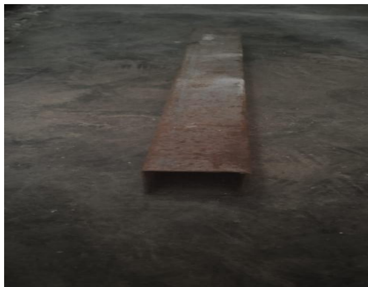
Gambar 3.4 besi hollow berukuran 40 mm x 40 mm tebal 2 mm
