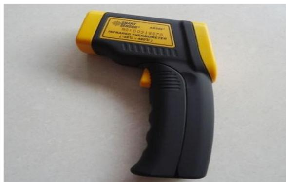
Gambar 3.13 Sensor Termoinfrared digital
