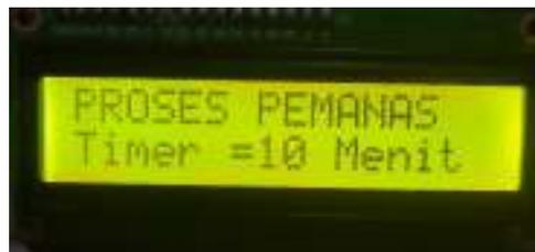
**Gambar 4.1.14** LCD 16x2 I2C
