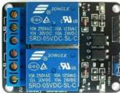
**Gambar 2.10** Modul Relay 2 Channel
