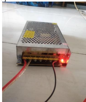
Gambar 2.9 Power Supply 12 VDC
