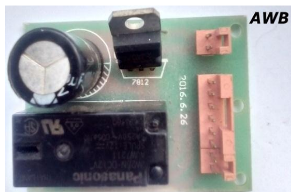
Gambar 2.29 Rangkaian Auto WindBack System
