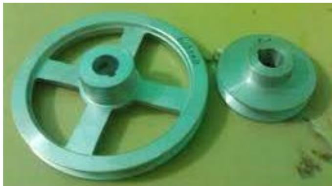
Gambar 2.4 Pulley tipe A
