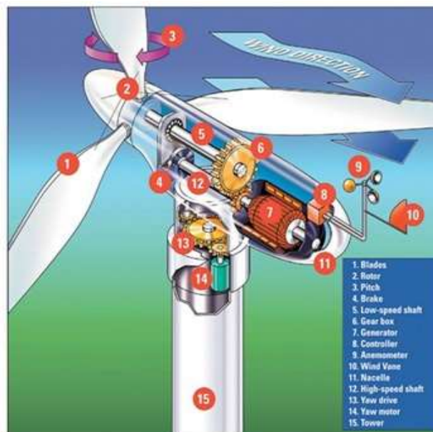
Gambar 2.9. Konfigurasi Turbin Angin Horizontal Axis (Abdul dkk, 2016)
