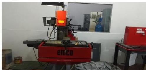
Gambar 3.3 Mesin Milling
