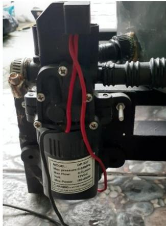
Gambar 3.4 Pompa Air DC 12 Volt
