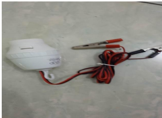
Gambar 2.13 Fitting inverter 12V to 220V
