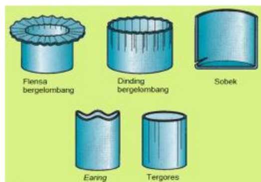
Gambar 2.12 Cacat ( Defect ) pada Hasil Deep Drawing . (Sumber: Groover, Mikell P., 2010, Fundamentals of Modern Manufacturing: Materials ,
