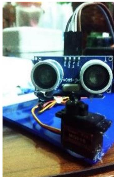
**Gambar 4.4 Sensor Ultrasonic**
