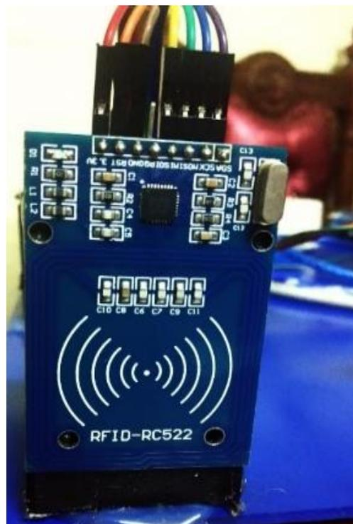
**Gambar 4.10** Sensor Radio Frequency
