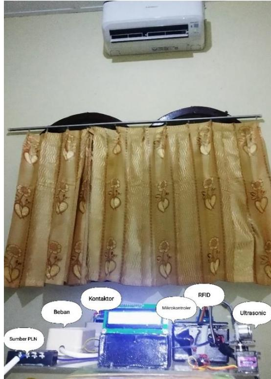
**Gambar 4.19 Proses Uji Coba Alat (Beban Pendingin Ruangan)**
