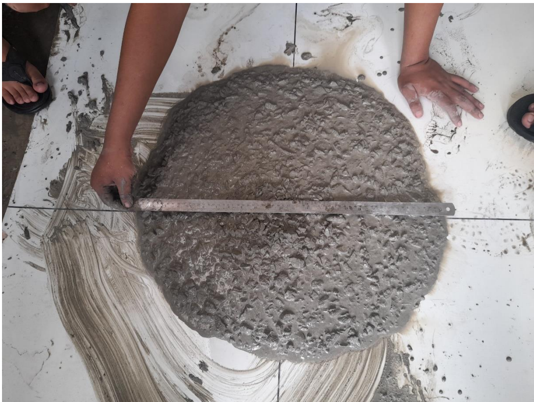
Gambar L.20: Pengukuran Diameter Slump Flow .
