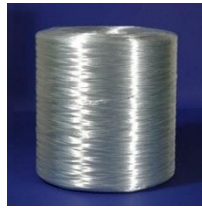
Gambar 2.3 Serat gelas roving
