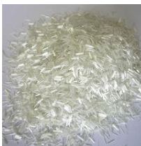
Gambar 2.5 Serat gelas chopped strand
