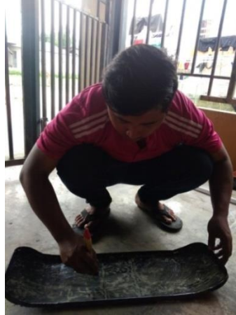
Gambar. 3.16 mengoleskan mirror glaze
