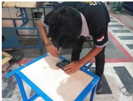
Gambar 3.24 Memasang Charger Controller
