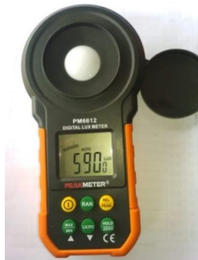
Gambar 3.10 Digital Lux Meter
