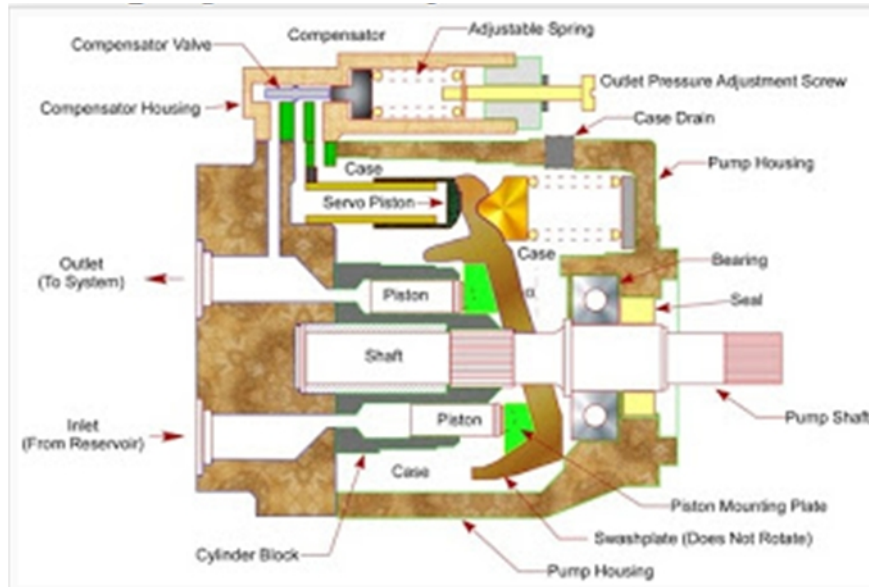
Gambar 2.4 Axial Piston Pump
