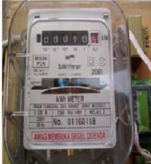
Gambar 2.5 KWH Meter Analog
