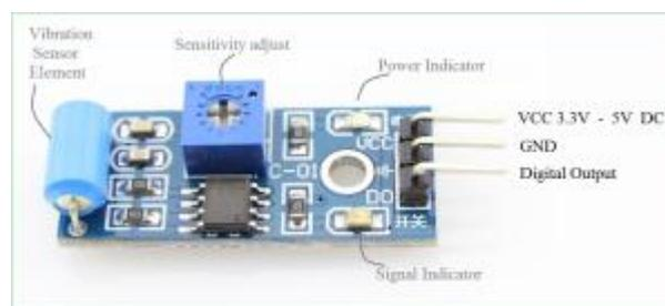
Gambar 2.14. *Vibration Sensor SW-420*
