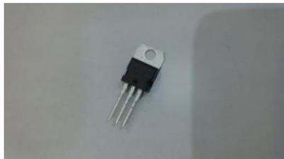
Gambar 2.11 IC Voltage Regulator
