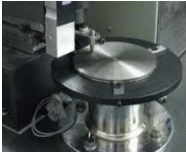
**Gambar 2.1** Tribometer *pin-on-disc*
