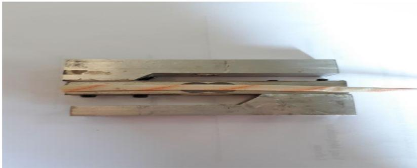
**Gambar 3.6** Sensor beban / Load cell
