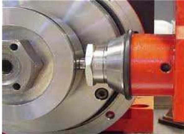
**Gambar 2.2** Tribometer *pin-on-ring*
