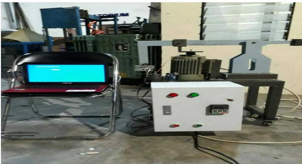
**Gambar 3.2** Alat Uji Tribology Pin-on-disc
