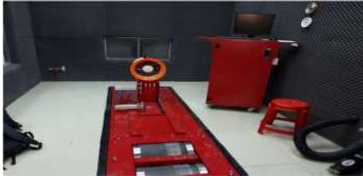
Gambar 3.6 : *Dynotest/Dynamometer*
