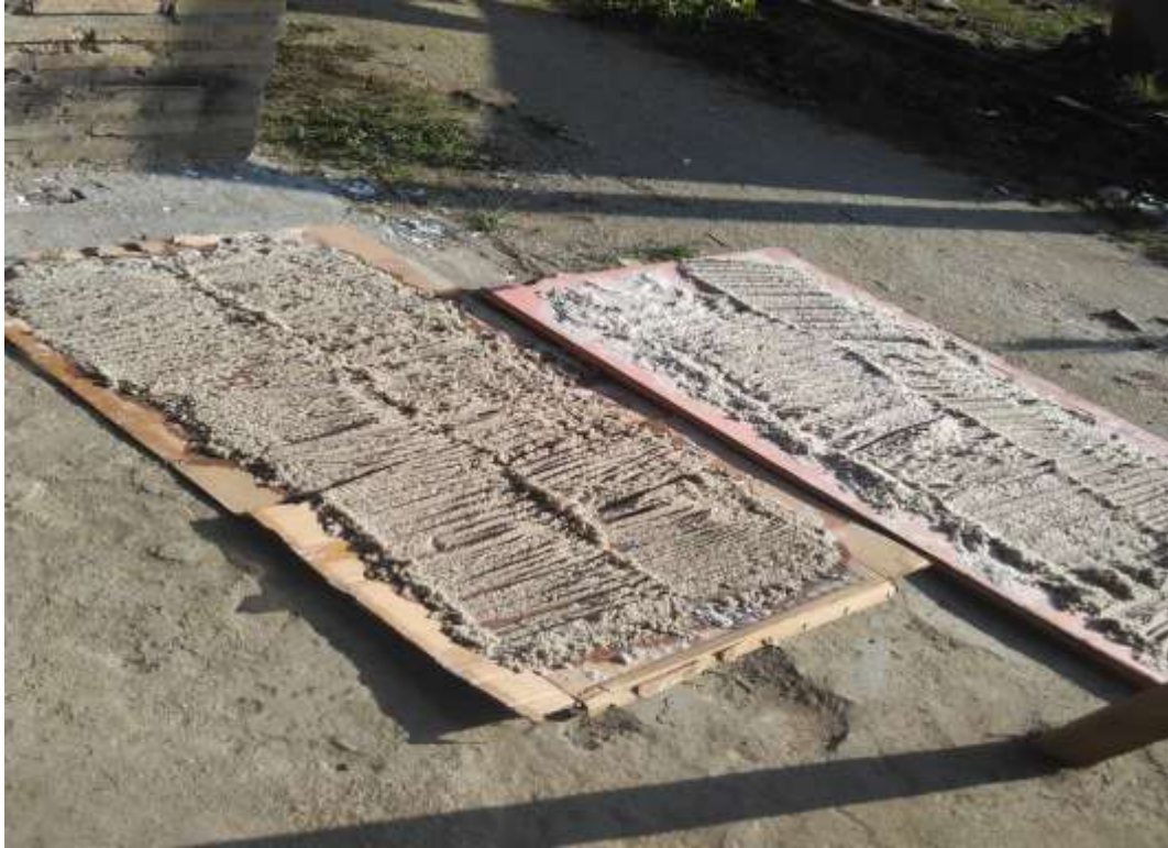
Gambar L5: Proses penjemuran pasir laut.
