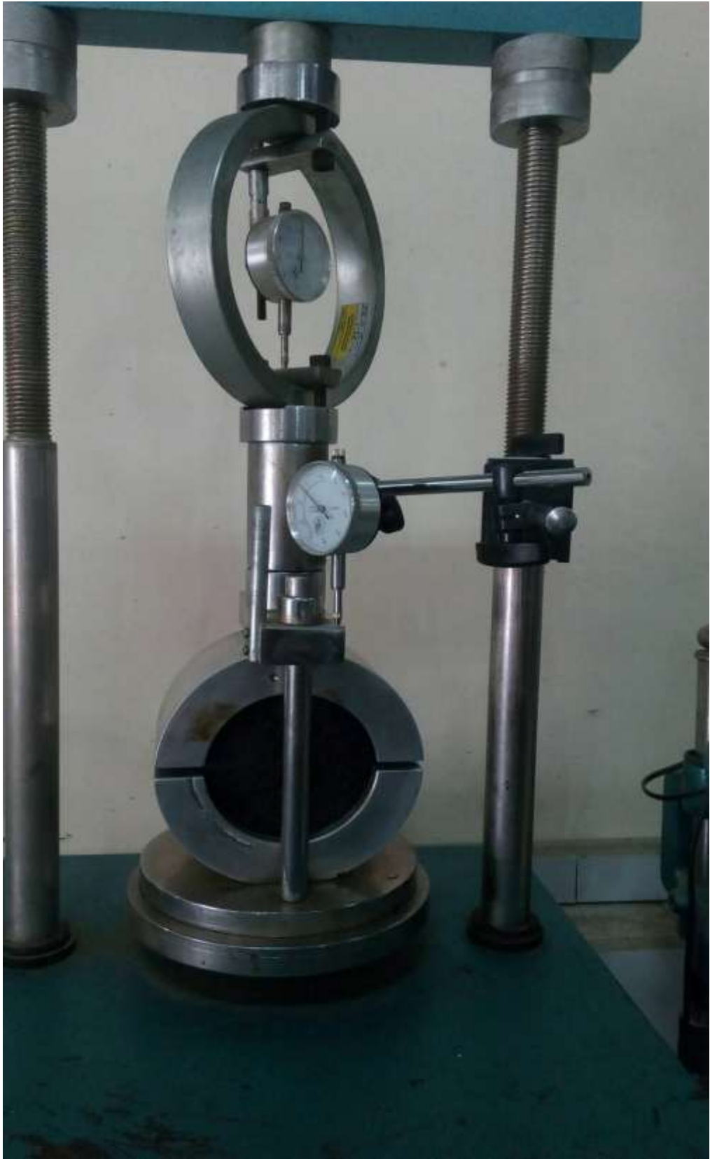
Gambar L13: Pengujian Marshall Test .
