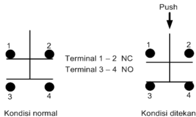
Gambar 2. 23 Prinsip Kerja Push Button Switch
