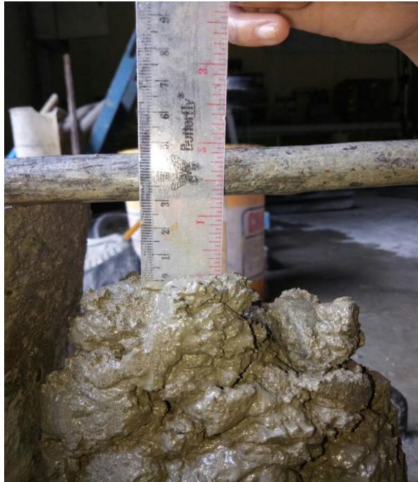
Gambar L7: Hasil pengujian slump test.
