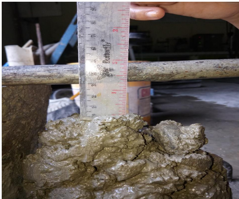
Gambar L8: Hasil pengujian slump test.
