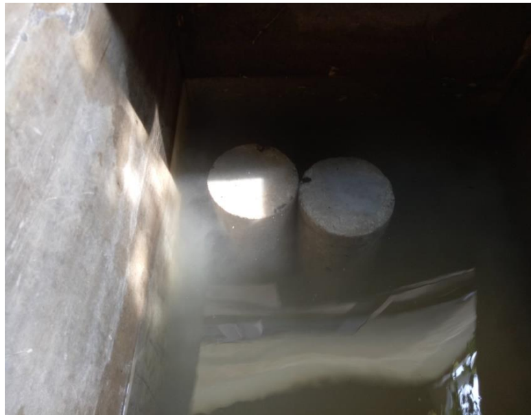
Gambar L10: Proses perendaman beton.
