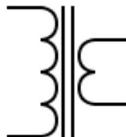
Gambar 2.18 Skema transformator step down
