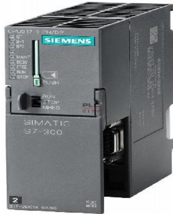
Gambar 2.10 PLC Siemens S7-300 CPU 317-2 PN/DP
