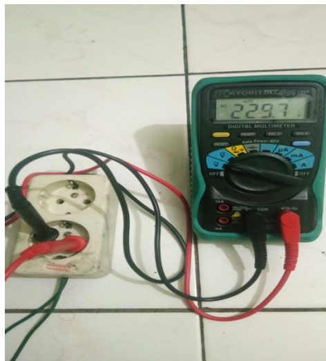
Gambar 3.14 Setting Pengukuran Output Inverter
