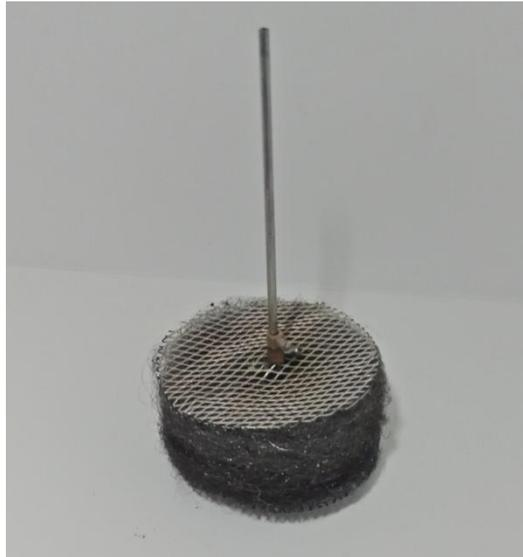
**Gambar 3.6** *Piston Displacer*
