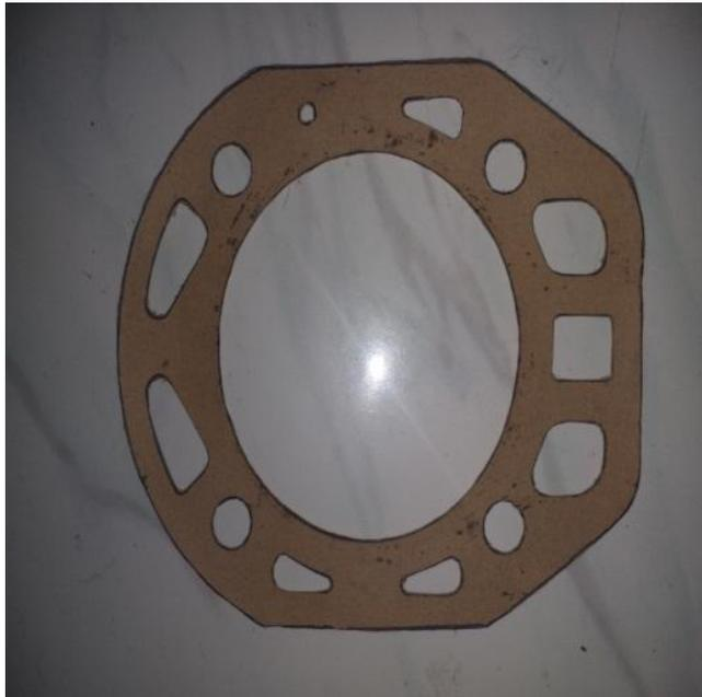
Gambar 3.2 Gasket *Head Cylinder*
