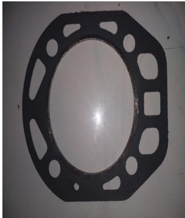
Gambar 3.3 Gasket *Head Cylinder* 1,80 mm
