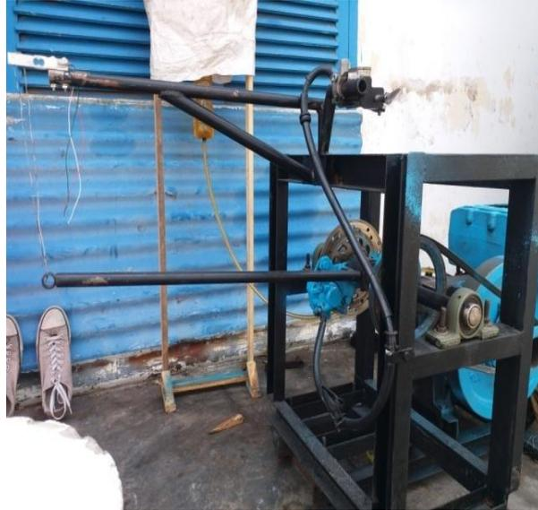
Gambar 3.9 Brake dynamometer
