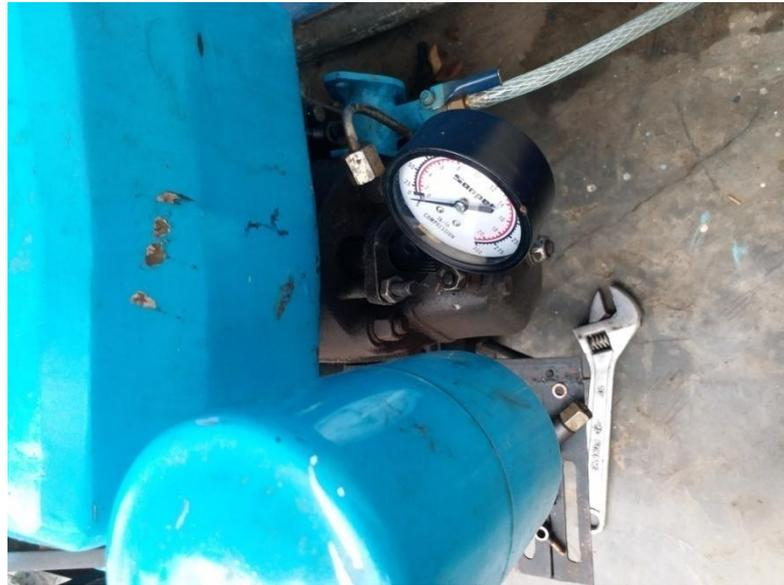
Gambar 3.19 Compression test
