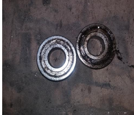
Gambar 3.2. Bearing fault (rusak)
