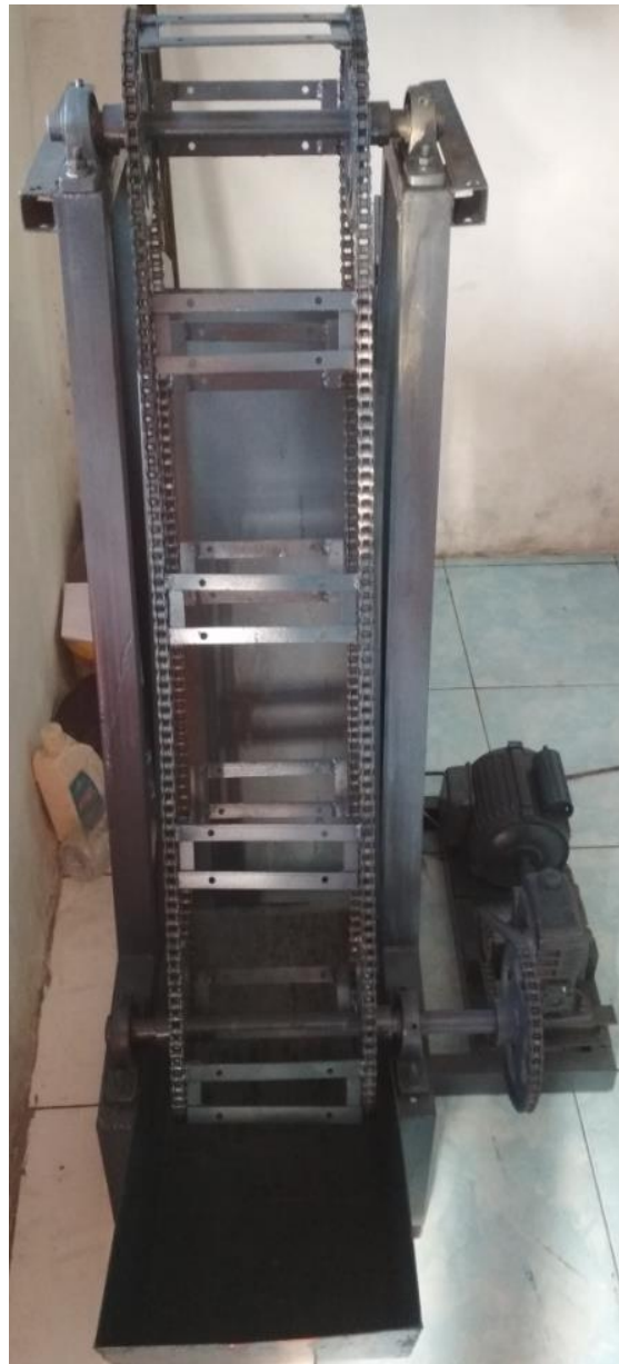
Gambar 3.13 Rantai Lintasan Elevator .
