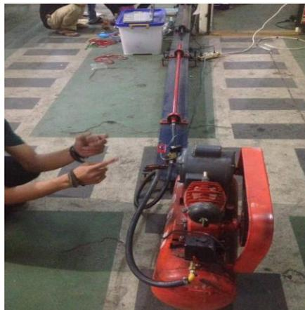
Gambar 3.6 Alat Uji Split Hopkinson Pressure Bar (SPHB)
