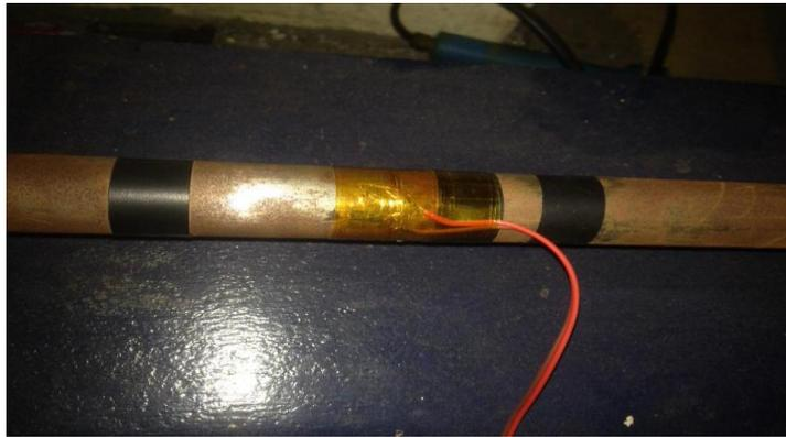
Gambar 3.38 Memasang *Strain Gauge*
