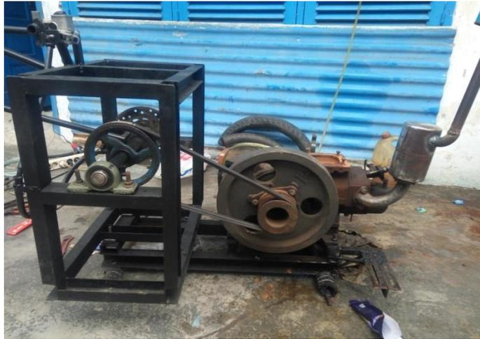
Gambar 3.21. *ChassisDynamometer*
