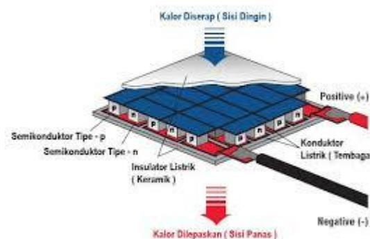
**Gambar 2.2 Skema Elemen Peltier**
