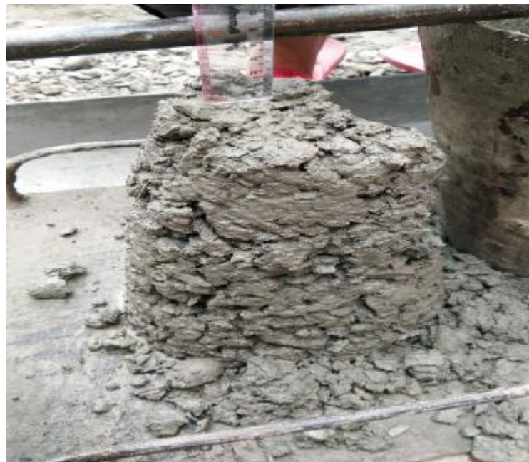
Gambar L10: Hasil pengujian slump test beton normal.
