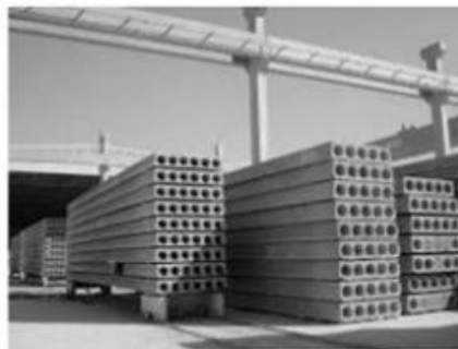
Gambar 2.3: PC voided slab .
