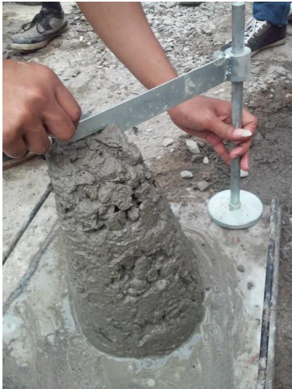
Gambar L7: Hasil pengujian slump test.
