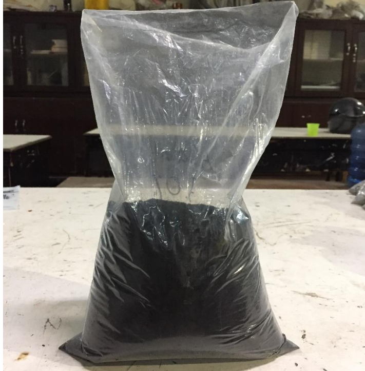
Gambar L.5: Crumb Rubber Lolos Ayakan No.100.
