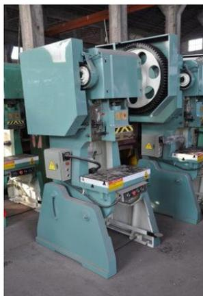
Gambar 2.3 Gambar Mesin Pres Mekanik (Klilmro, 2018)
