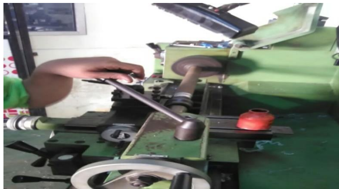
Gambar 3.31. Membubut besi AS (poros)
