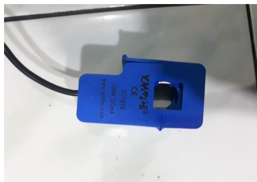
Gambar 3 : sensor arus STC013-030
