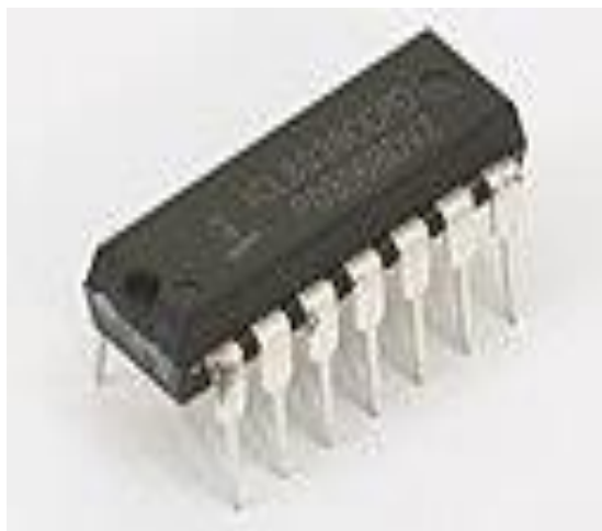
Gambar: 2.6 Integrated Circuit 8038 (commons wikimedia.org)
