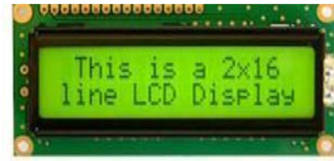
Gambar 2.10 LCD 2x16
