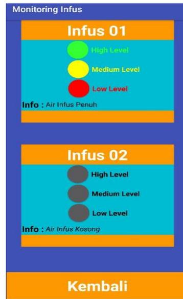
**Gambar 4.7 Kondisi Cairan Infus Pada Posisi *High Level***
