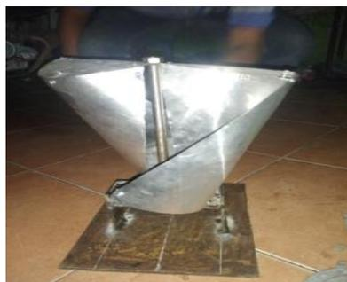
Gambar 3.6 Model turbin angin type Sudu Heliks
