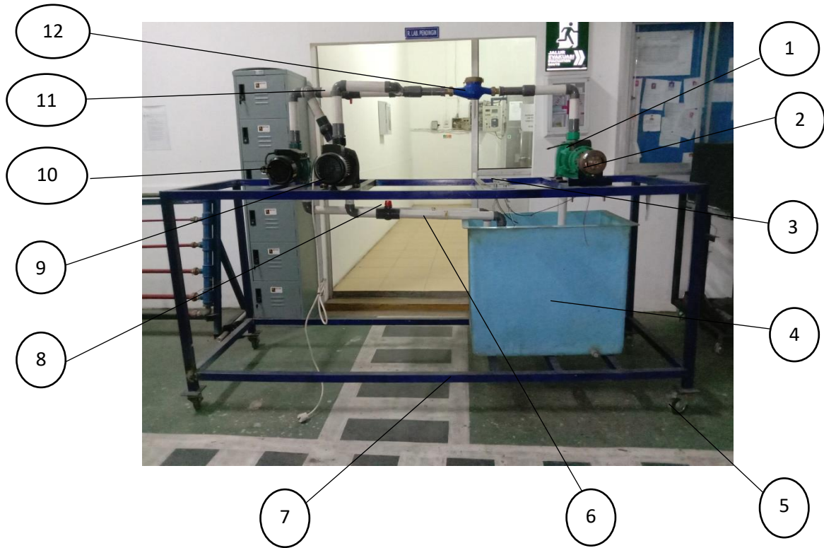
Gambar 4.1. Bagian-Bagian Pump As Turbine (PAT)
