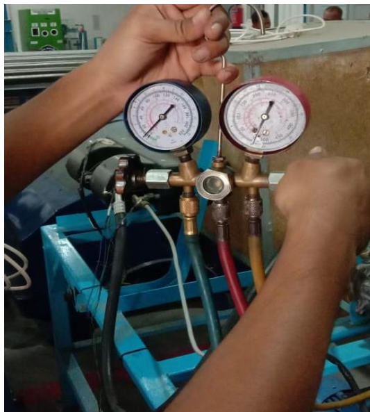
Gambar 4.9 Membuka katub HP manifold gauge
